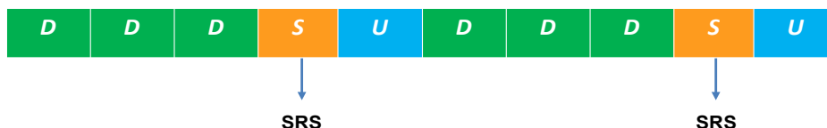
Figure 8: TDD frame structure
